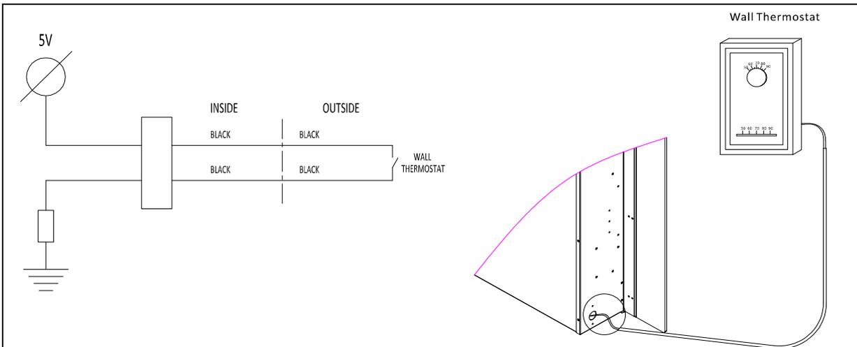
NOTE: THE WALL THERMOSTAT WILL WORKING WHEN THE HEATER ON TEMP. SETTING.PLEASE REFER TO THE MANUAL CONTROL AND THE REMOTE CONTROL.
