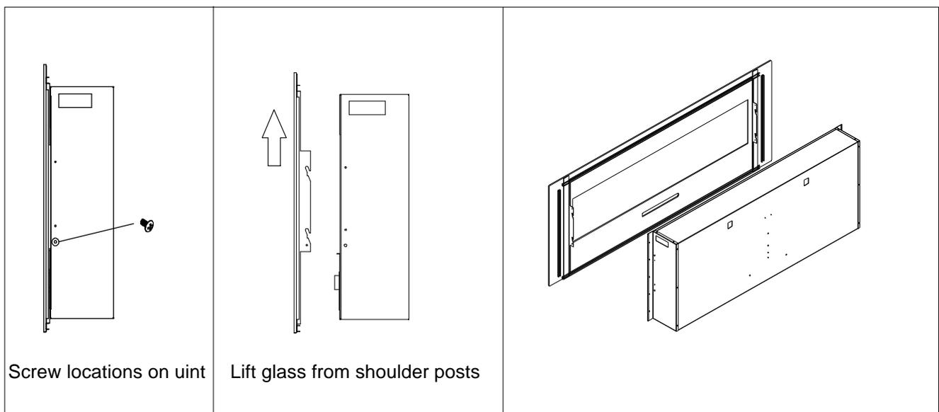
3. To replace the glass, lift onto the 4 shoulder posts. For a Wall Mount installation, replace the two or four screws to secure the glass. For Flush Mount installs it is not possible to replace the screws.
