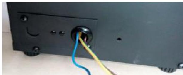
3. Return the cover plate to the left side and screw the two screws back in to fasten the plate.
